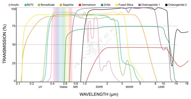
Thickness Considerations: Band transmission % is not usually affected significantly by thickness. However, the transmission bandwidth often narrows dramatically as thickness increases.
